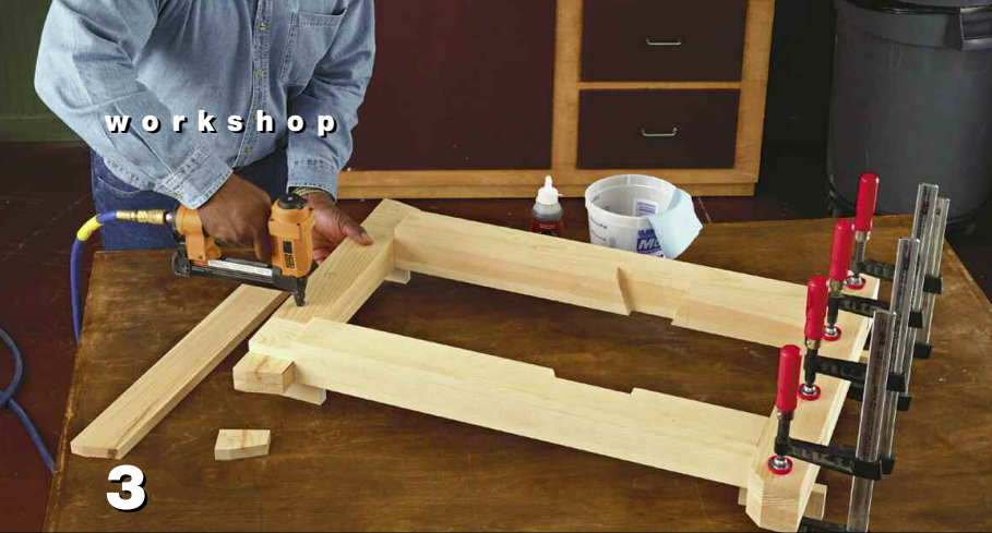
3 Carefully line up the laminations when gluing the feet and top rails to the legs. Glue and staple one piece in place at a time, and then clamp the entire assembly.
