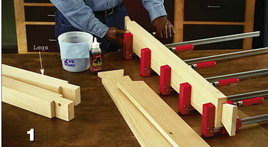
Glue the stretcher parts together, lining up the ends of the inner stretcher with the dovetail shoulders that you cut on the outer stretcher. Spread a thin layer of glue on one face, and use a damp cloth to wet the mating face.
