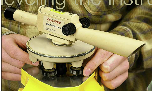
Align the sight with one set of screws. Turn the screws evenly to level the sight.
