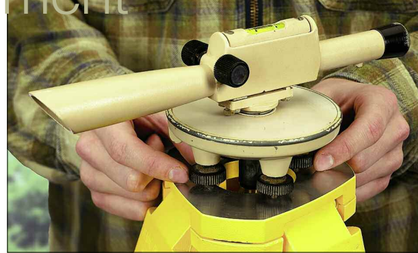
Turn the sight to align with the second set of screws and adjust for level again.
